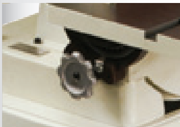
LARGE LOCKING NUT AND TABLE ANGLE SCALE
