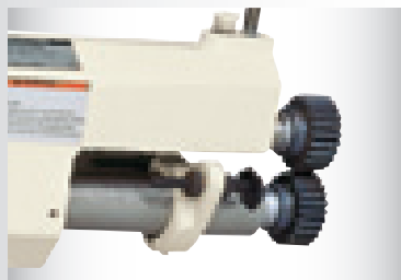
SIX INTERCHANGEABLE ROLLS FOR BEADING, CLOSING, TURNING, JOGGING, CRIMPING AND FLANGING
